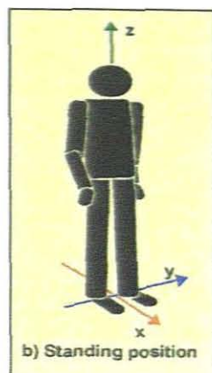
Figure 1: Co-ordinate system used during the measurement of Whole body vibration inside offices.
