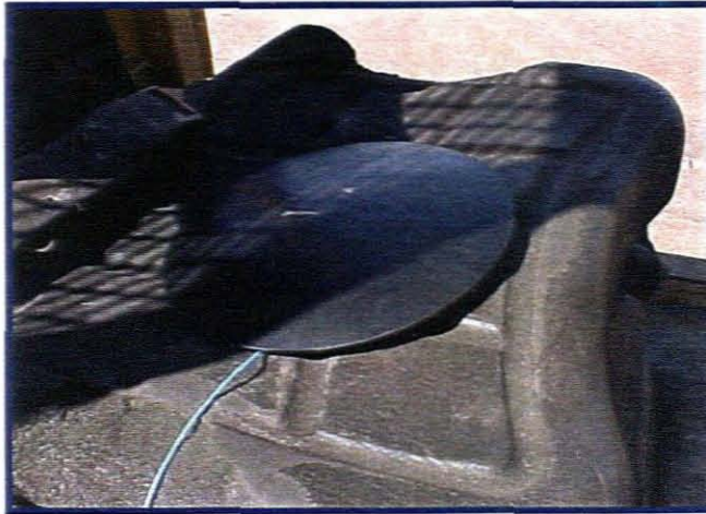
Figure 8: Vibration Seat Pad Used During Whole Body Vibration Measurements
