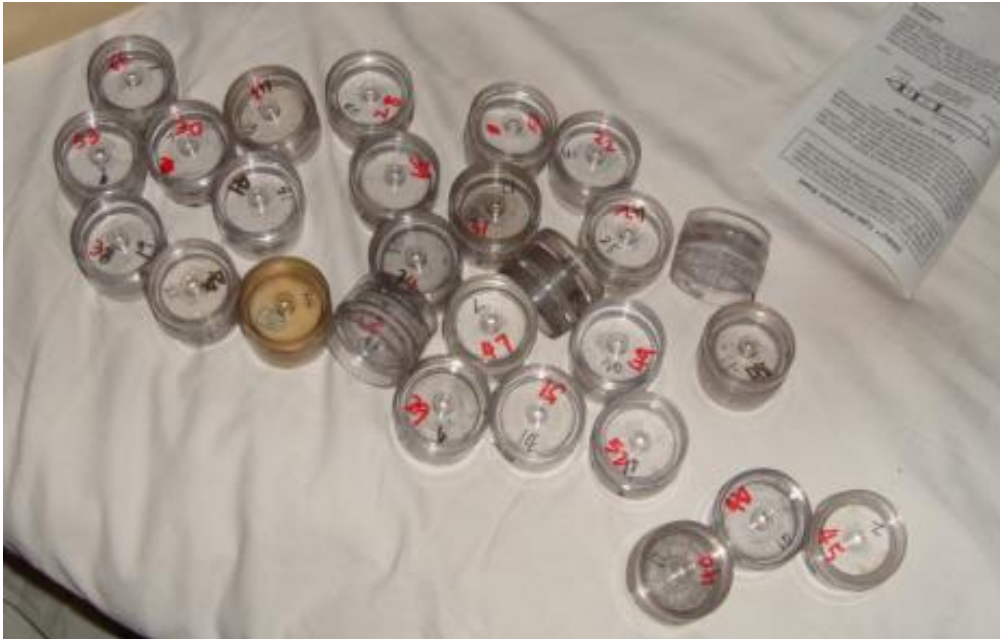
Figure 3.7 Filter. PTFE-laminated membrane filter, 2- \mu m pore size, 37-mm diameter in cassette filter holder
