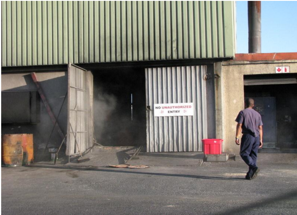
Figure 4.36: Fugitive bottom ash blown into the environment
