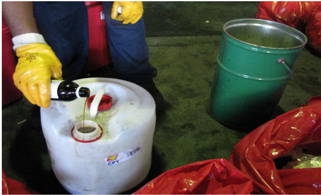
Figure 4.40: Indiscriminate mixing of liquid pharmaceutical waste prior to incineration
