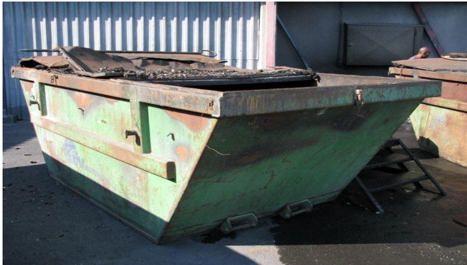
Figure 4.38: Open-lidded skip containing cold bottom ash
