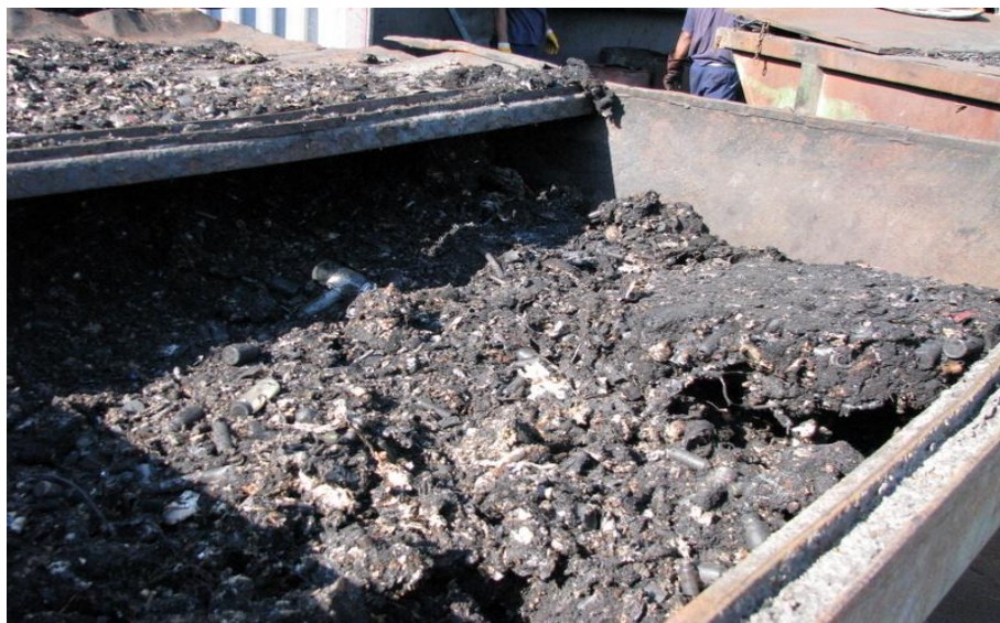
Figure 4.39: Bottom ash partially combusted
