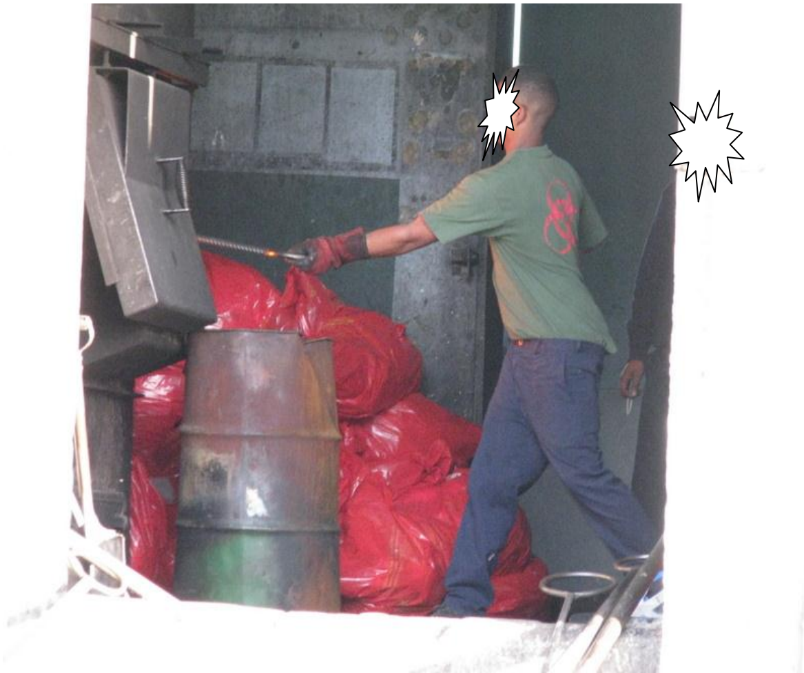
Figure 4.35: Improperly clad workers removing bottom ash
