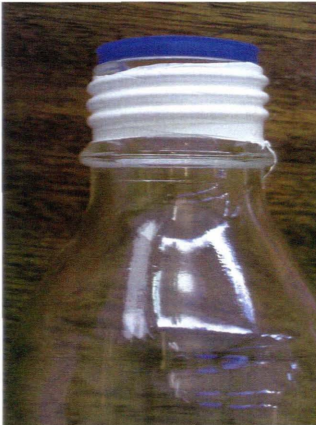
Fig. 2.4: Teflon seal around Schott bottleneck thread.
