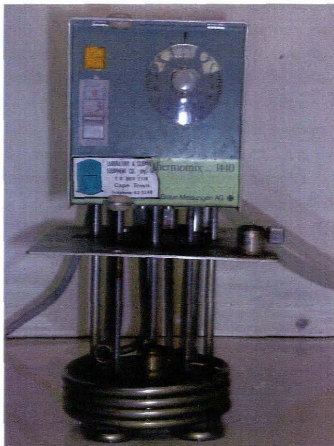
Fig. 2.3: The Thermo Mix 1440, Braun Melsungen AG (Germany) pump used for circulating cooling water ( 10^{\circ}\text{C} ) through glass cooling jackets
