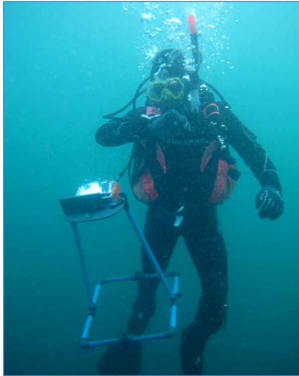
Figure 2.2: SCUBA diver, within the study area, with photo-quadrat utilised for image capturing (Photo by: Marco Worship 2012)
