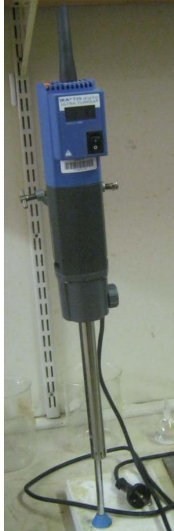
Figure 3.2 Ultra-Turrax® T25 homogenizer
