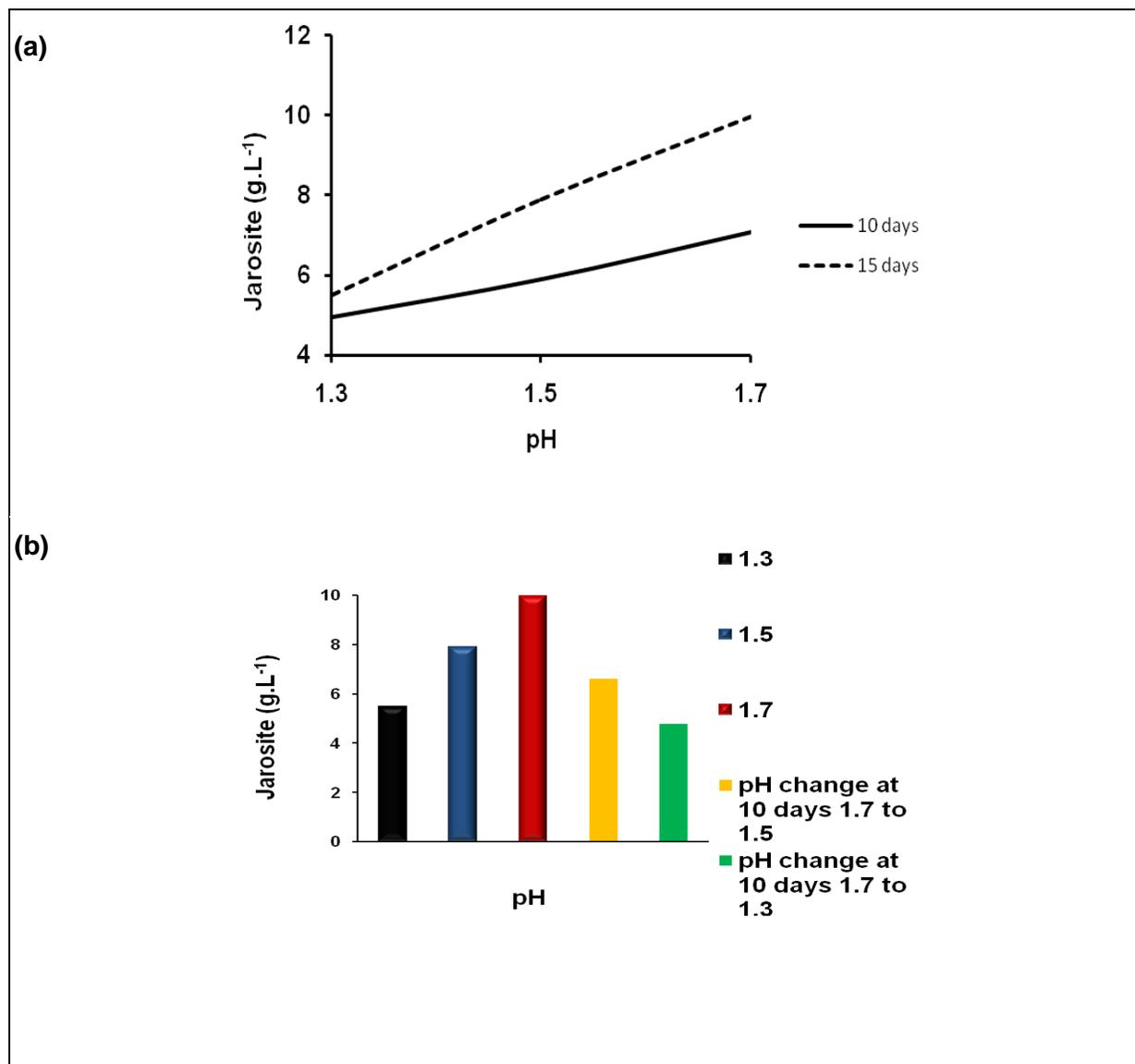
**Figure 4.1:** Variation of jarosite precipitate accumulation versus bioreactor solution pH after (a) 10 and 15 days of continuous operation. (b) 15 days of operation at constant pH compared to the variation when pH was lowered to 1.5 and 1.3 after 10 days for additional five days of operation.
