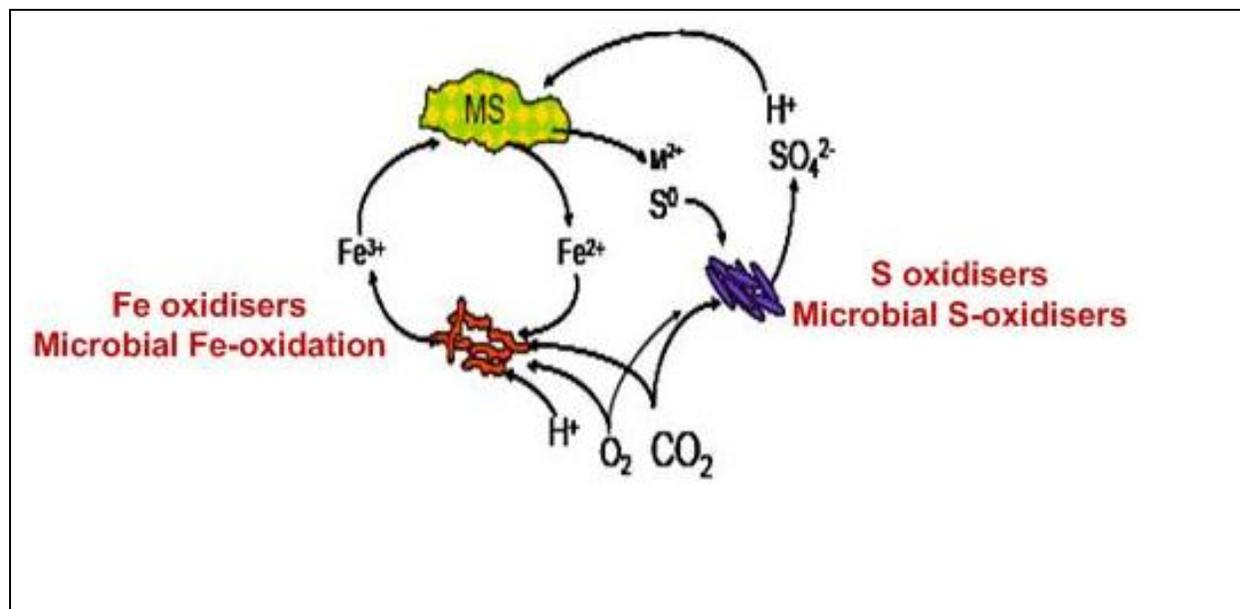
**Figure 2.1:** A schematic representation of the mechanism of bioleaching (Breed and Hansford, 1999c) (Hansford and Vargas, 2001)
