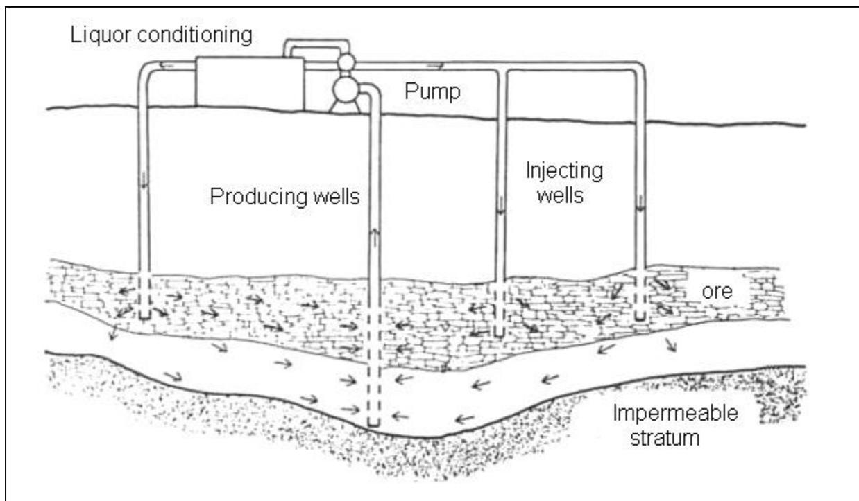
**Figure 2.5:** Schematic drawing showing bioleaching of the low grade mineral sulphide ore using the in-situ method
