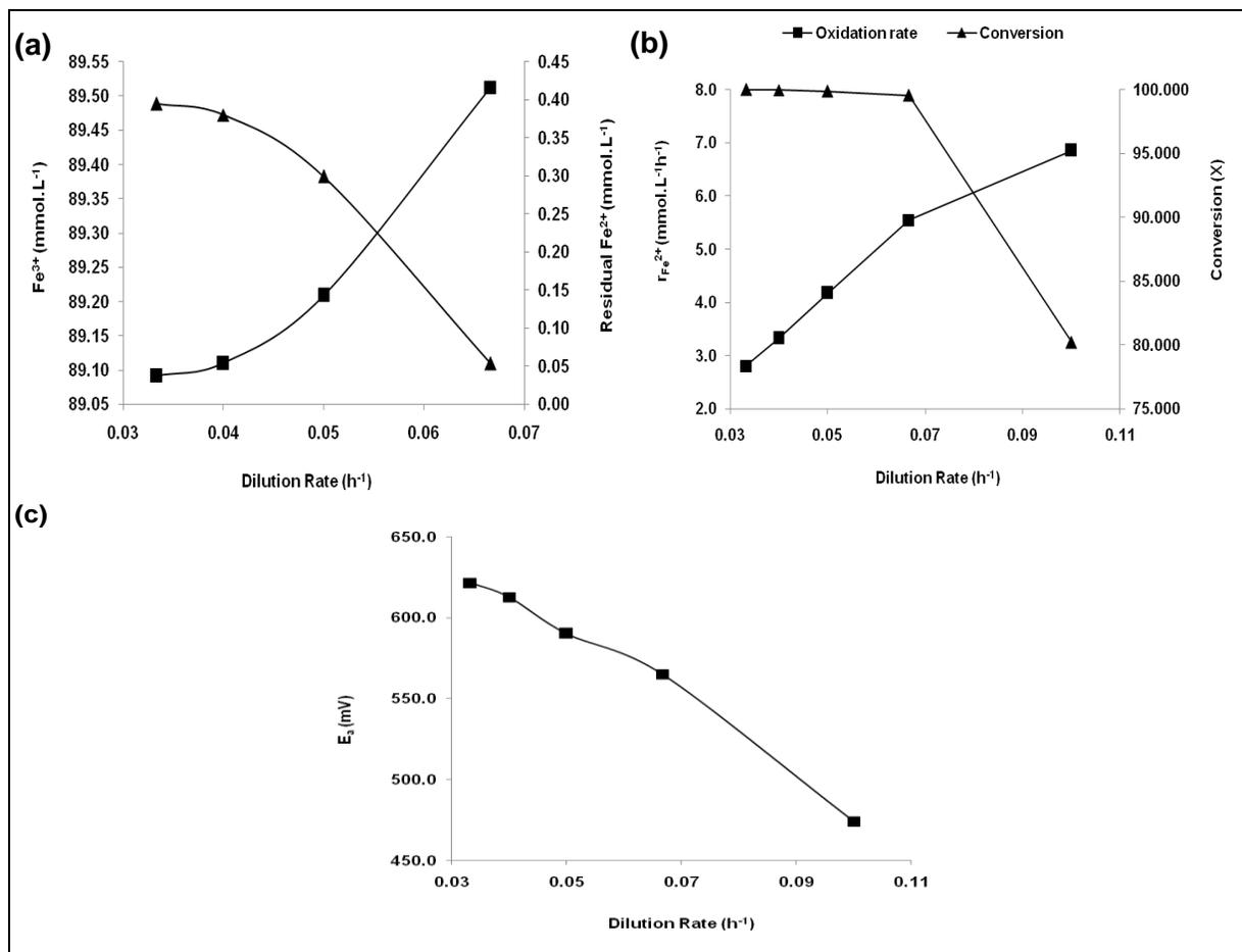
**Figure 4.2:** Dilution rate versus (a) iron species (ferric-iron and residual ferrous-iron); (b) ferrous-iron oxidation and conversion; (c) solution redox potential (Ag/AgCl)
