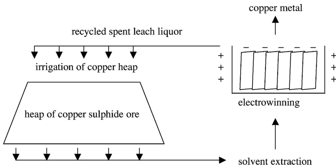
**Figure 2.3:** Schematic diagram showing the flow of the leaching liquor in bioleaching of low grade copper sulphide ore using the heap method (Rawlings, 2002).
