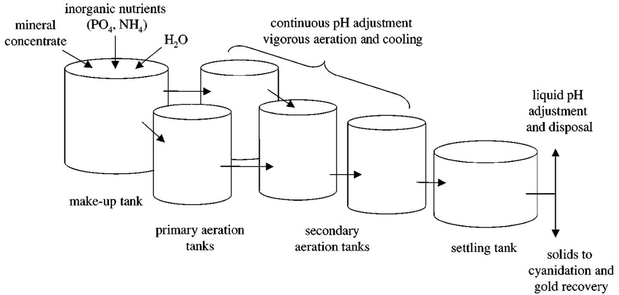
**Figure 2.4:** Schematic diagram showing the flow of materials between stirred tanks in the pre-treatment of gold from the arsenopyrite concentrate using the microorganisms in the stirred tank system (Rawlings, 2002)
