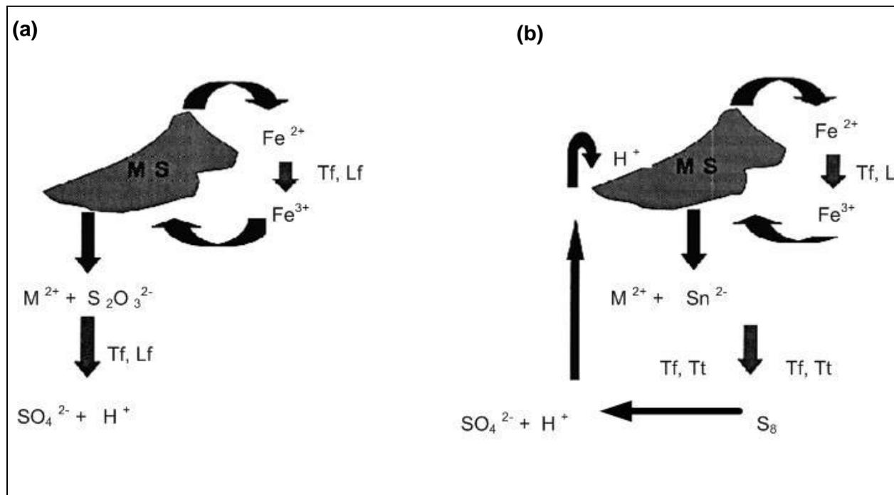
**Figure 2.2:** (a)thiosulphate and (b)polysulphide bioleaching of the sulphides minerals (Schippers& Sand, 1999)
