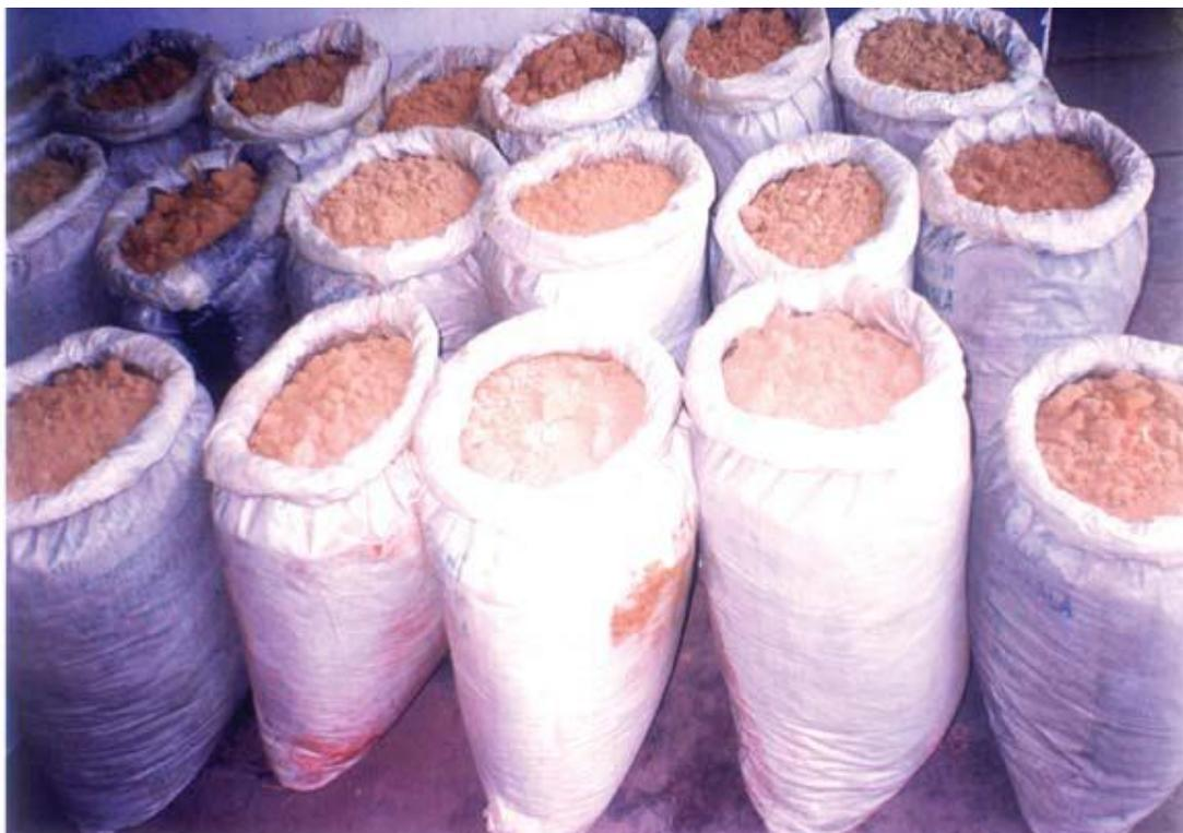
**Figure 2.7:** Jarosite produced from the Debari Zinc Smelter plant, Rajasthan, India (Pappu *et al.*, 2006).
