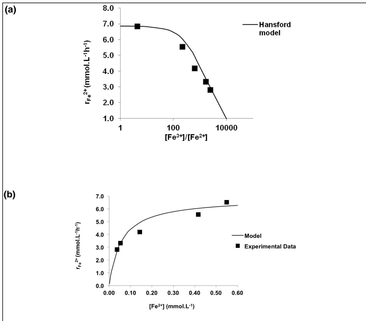
**Figure 4.3:** (a) The fit of rates data to the Boon and Hansford model, Equation 2.18 (b) the ferrous-iron oxidation rate versus residual ferrous-iron in relationship to the trend of the Monod model, Equation 2.19.
