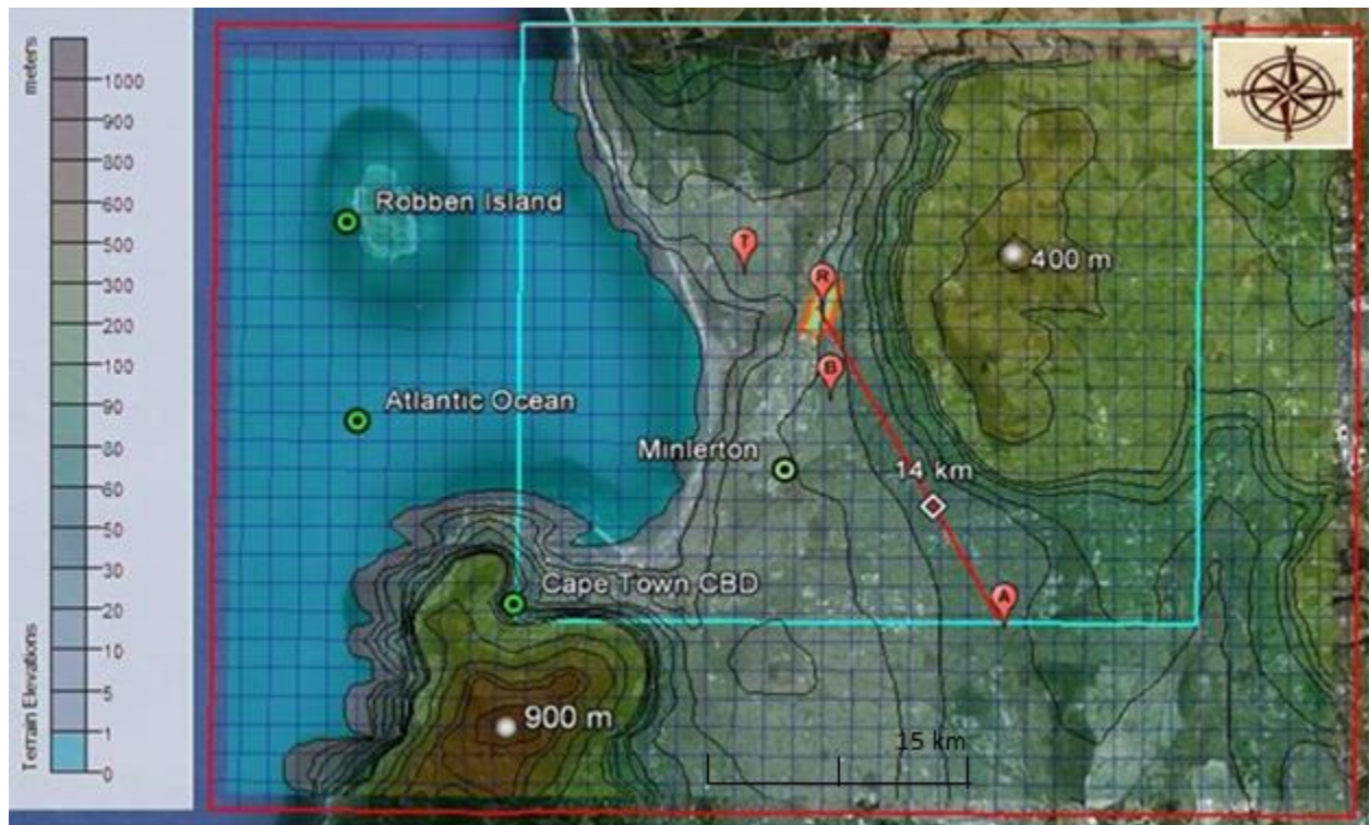
Figure 7: Study area for CALPUFF (red boundary) and AERMOD (blue boundary) with receptor grid, location of refinery (R), monitoring stations (T, A, B) and surrounding communities.
