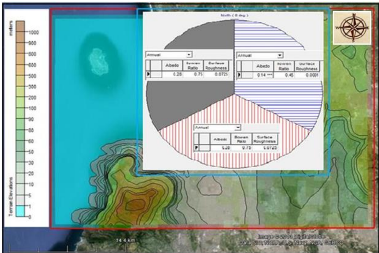
Figure 23: Sectors and Surface Parameters used in AERMET run.
