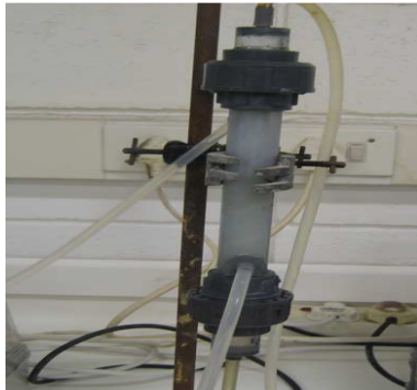
Figure 3.3: A Counter-current, double pipe Perspex bench-scale reactor
