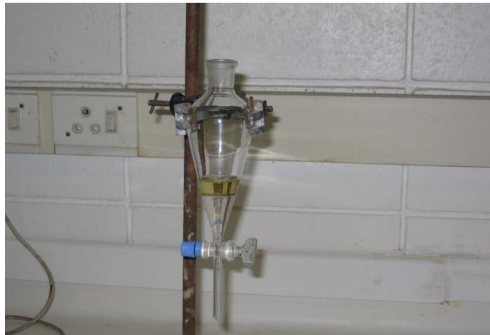
Figure 3.5: The separation process for the solvent and the feed solution
