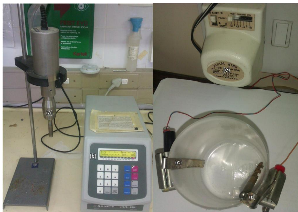
Figure 4. 4: Electro-physico-chemical assisted adsorption: (a) - sonicator probe, (b) - sonicator controller unit (Sonic & Materials Inc, USA), (c) - anode, (d) - cathode and (e) – electrical current adapter
