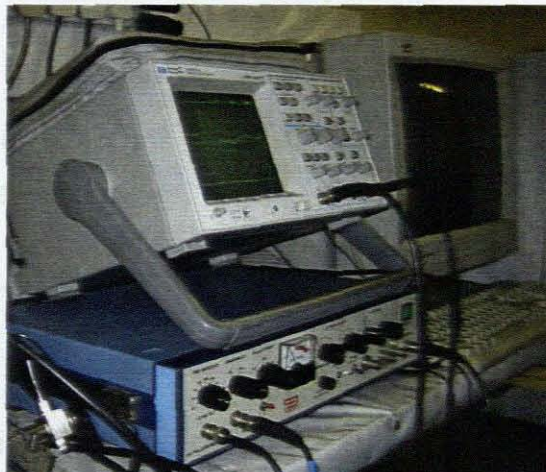
Figure 4.4: A photograph of the ultrasonic equipment used in the study, showing the Panametrics 5058PR pulser-receiver under the HP 54602B oscilloscope and a computer on the far right.
