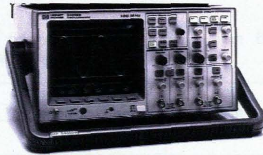
Figure 4.6: Photograph of the Hewlett Packard 54602B oscilloscope.
