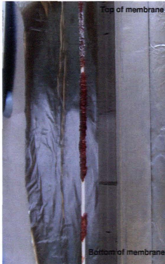
Figure 6.4: A ceramic membrane showing biofilm sloughing during operation of the SFMGR system
