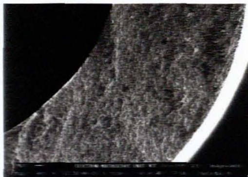
(a) Cross section of a 3 mm x 2 mm ceramic membrane (Magnification of 400x)
