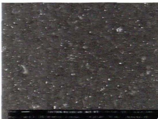
(d) The inside surface of the 40 nm inside coating of \alpha\text{-Al}_2\text{O}_3 (Magnification of 2000x)
