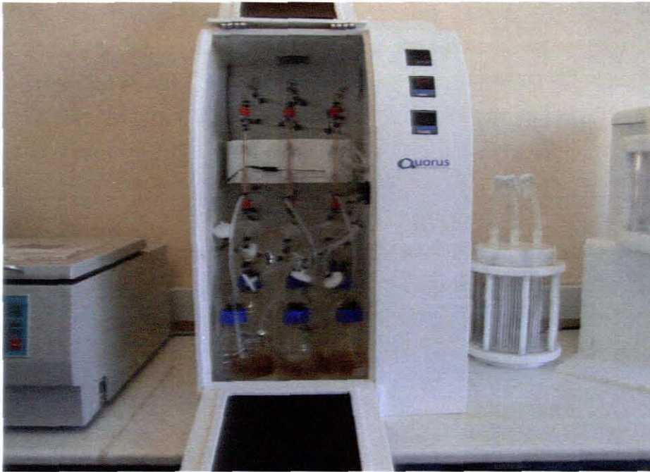
Figure 3.1: Photograph of the 1 x 3 SFMGR Quorus rig constructed of white Corian plastic
