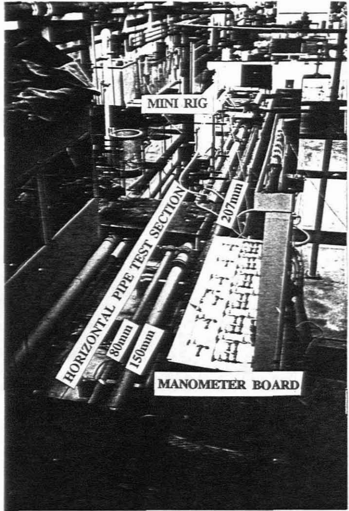
Figure 3.4: Horizontal test section
