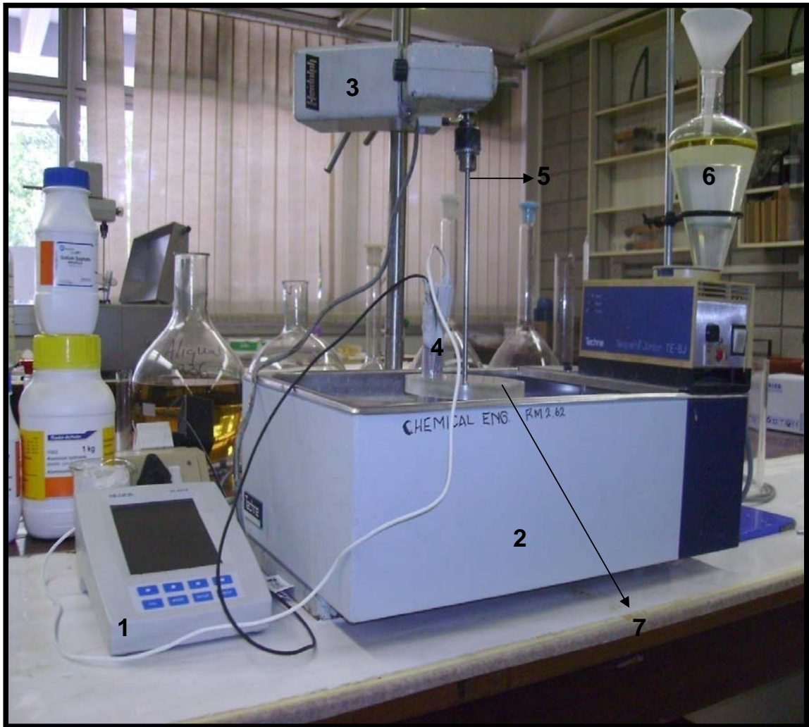
Figure 3.3: Solvent extraction experimental set-up: (1) pH meter Hanna HI 4212 (2) Thermostated water-bath (3) Heidolph variable speed overhead stirrer (4) Probes Hanna HI 1053B-1 and Hanna HI 7662-T for pH and temperature measuring, respectively (5) Flat-blade turbine double stirrer (6) Separating funnel (7) Batch reactor
