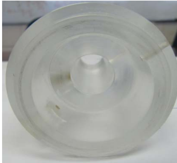
Figure 3.4 Photograph of a long (tube) square-edged orifice
