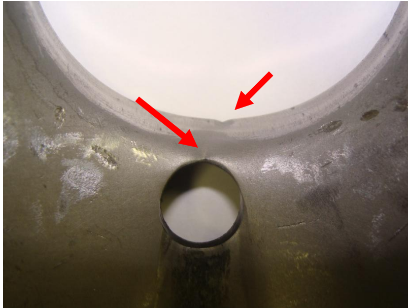
Figure 20.4: Component excessive plastic straining in an unacceptable condition
