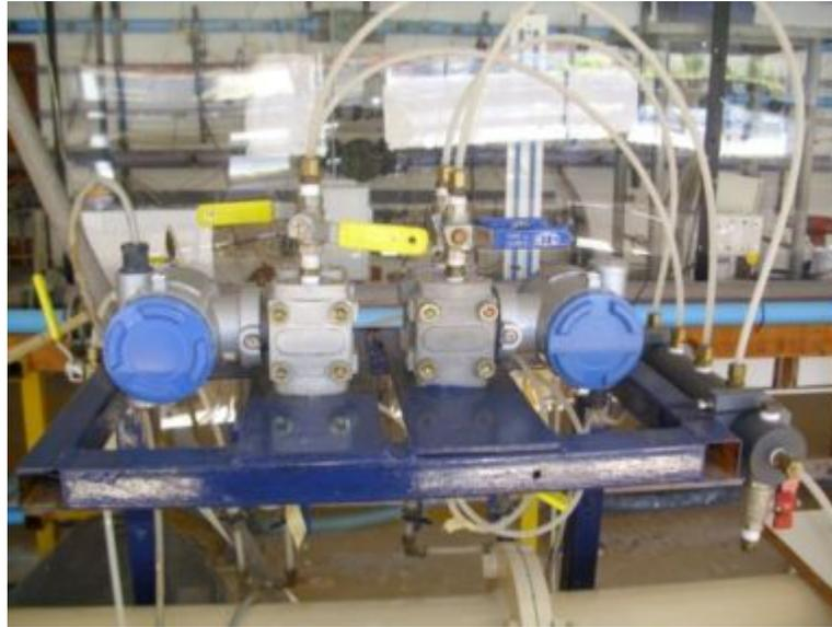
**Figure 3.5: Differential Pressure Transducers (DPTs)**
