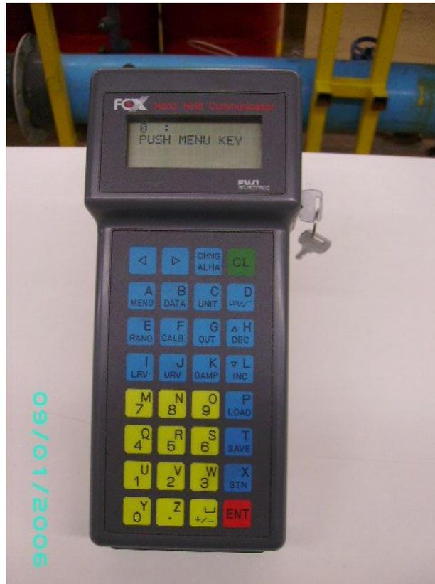
Figure 3.7: Hand-Held Communicator (HHC)
