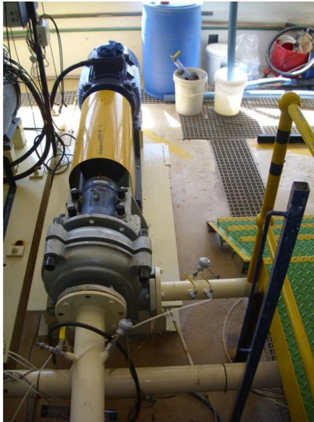
**Figure 3.3: Warman 4/3 centrifugal pump**
