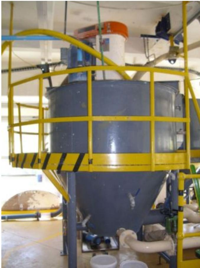
Figure 3.2: Mixing tank
