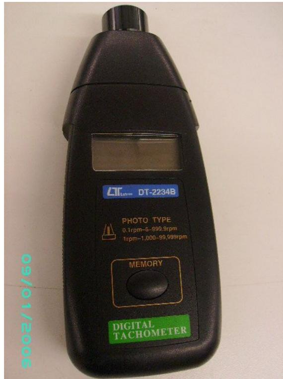
Figure 3.8: Tachometer
