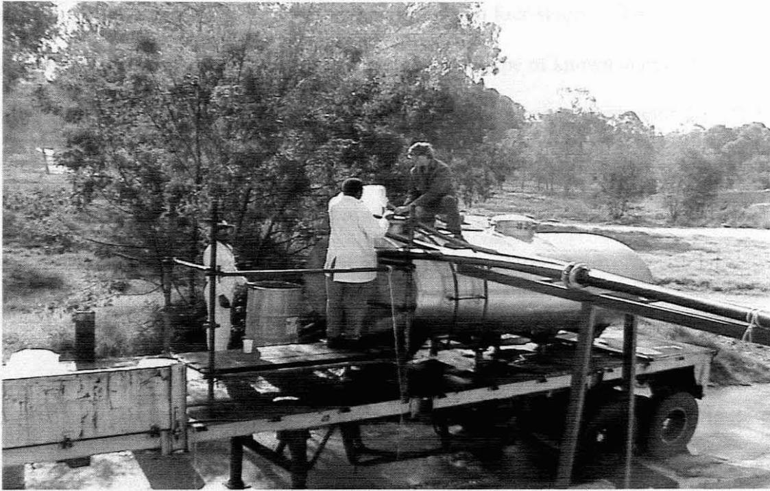
FIGURE 3. 1 Receiving tanker acting as a discharge reservoir.
