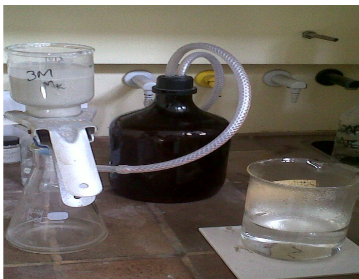
Figure B.1: Filtration of activated clay and washing with hot distilled water
