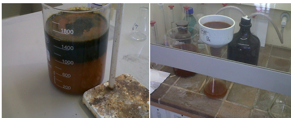
Figure B.2: Formation of ZVINPs just during titration and stabilisation of ZVINPs under fume cupboard
