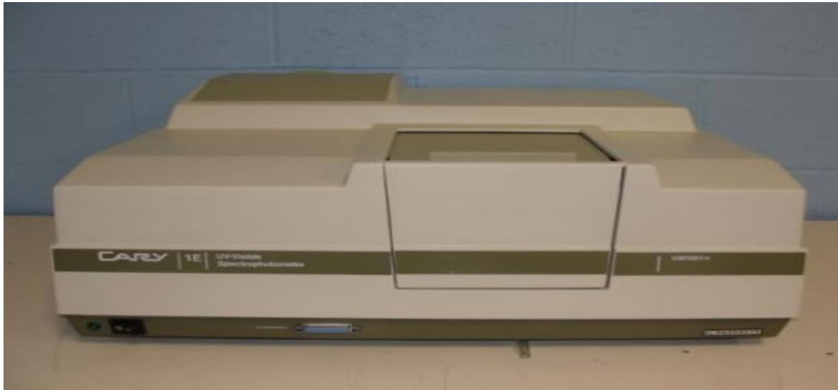
Figure 3.4: Spectrophotometer used for ammonia analysis (CPUT, Food Technology, 2012).
