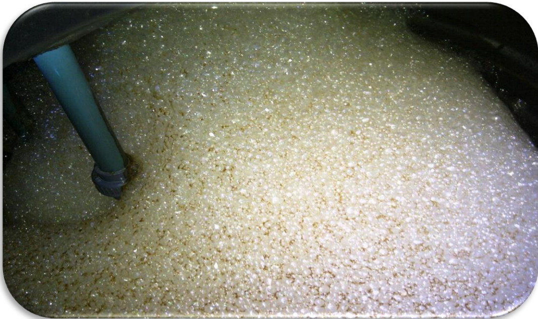
Figure 4.5: Foam formation in the holding tank
