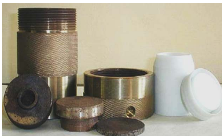
Figure 2.7 A typical pressure vessel/autoclave (Byrappa, 2005)
