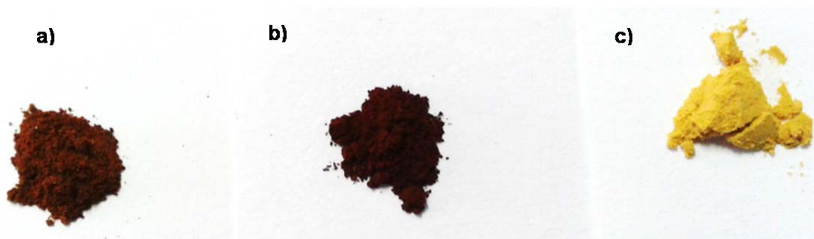
Figure 6.6 Colour of different iron oxides produced using different iron anions, in a) \beta -FeOOH particles from \text{Cl}^- , b) \alpha - \text{Fe}_2\text{O}_3 from \text{NO}_3^- and c) \text{H}_3\text{O} \cdot \text{Fe}_3(\text{SO}_4)_2(\text{OH})_6 from \text{SO}_4^{2-}
