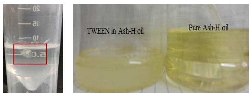
Figure 4.4: An AN solution (60 wt%) containing 1 wt% Tween 80 surfactant, (left) and dispersing of Tween 80 in pure Ash-H oil (right). Squares in left picture indicate the formation of Tween 80 agglomerates in the aqueous phase
