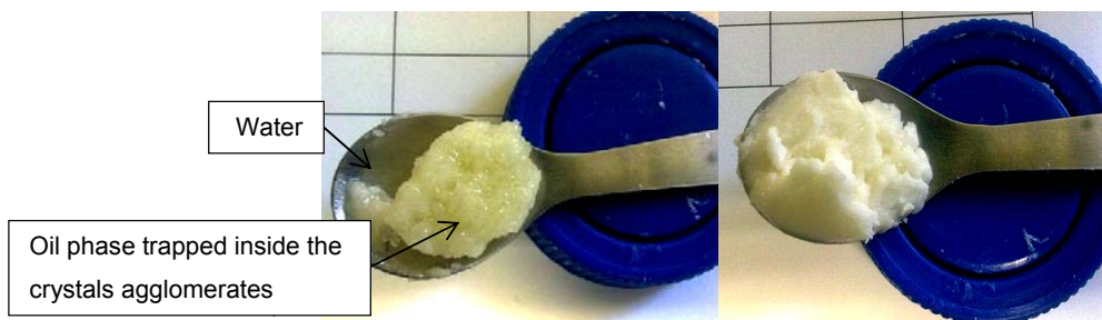
Figure 5.35: The white creamy paste structure of fully crystallised PIBSA-Mea/Spans emulsions (right) and the phase separated structure including AN agglomerates of the fully crystallised PIBSA-Mea/Tweens emulsions (left)
