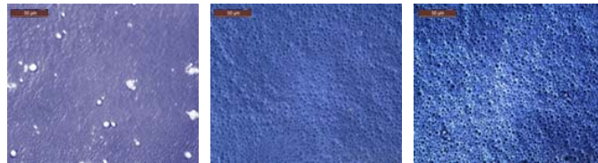
Figure 4.9: Photomicrographs of pumped emulsions stabilised by the PIBSA-Mea only (left), PIBSA-Mea/Span 80 (middle) and PIBSA-Mea/Tween 80 (right). Scale bar, 50 \mu\text{m} = 6 mm
