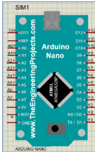
Figure 4.32: Arduino Nano Microcontroller on Proteus simulation platform
