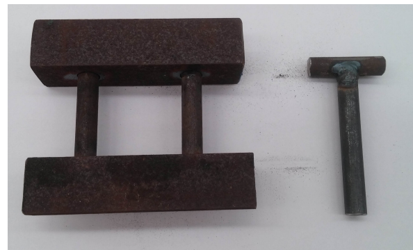
Figure 3.44: Bend Test jig for the composite sample testing.
