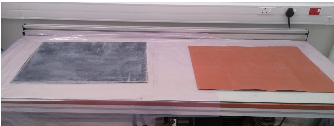
Figure 4.129: Carbon Fibre material with the adhesive layer applied and the prepared FR4 backed copper foil layer prior bonding.
