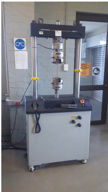
Figure 3.43: The newer tensile test machine available at the engineering lab.
