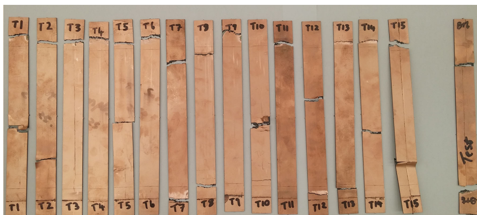
Figure 4.111: Material test specimens after tensile testing.
