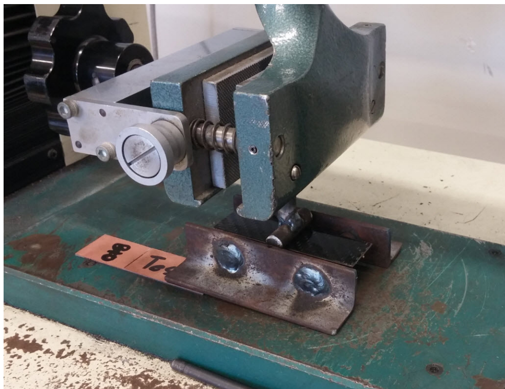
Figure 4.114: Bend test sample in the testing machine.
