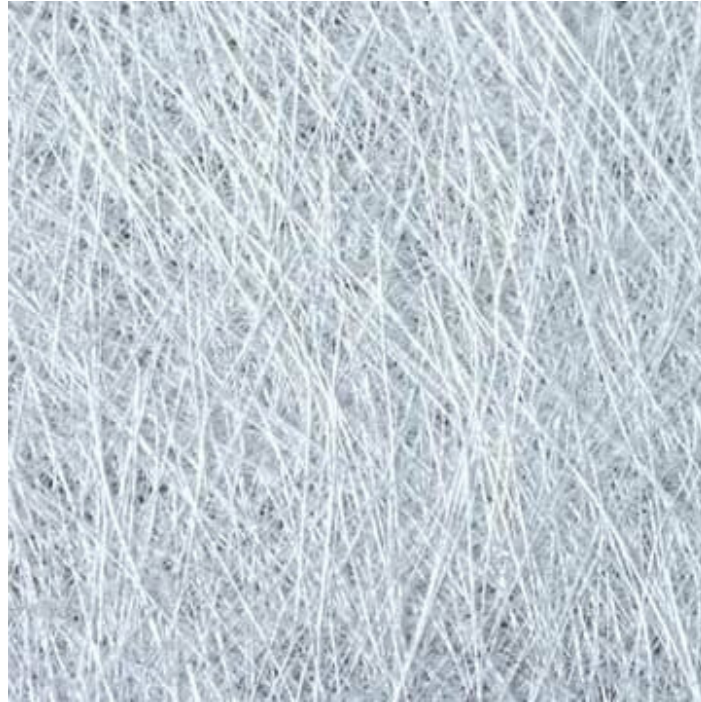
Figure 2.7: Chop-strand mat. (AMT-Composites, 2015)
