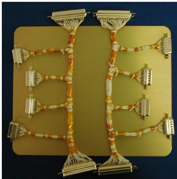
Figure 2.17: Aluminium panel with conventional type wiring harness attached. (DiPalma et al., 2004)
