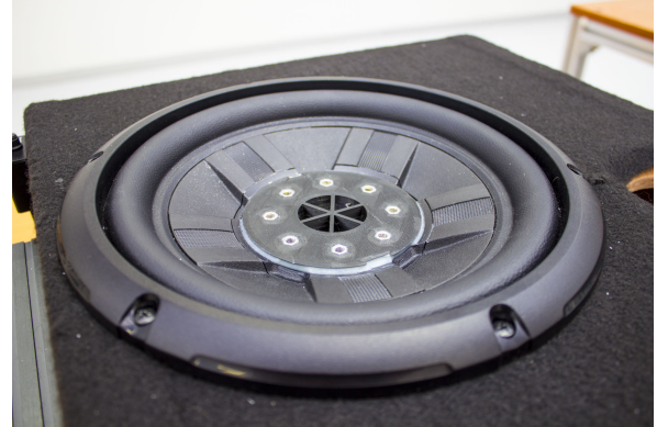
Figure 3.46: Closer view of the bonded mounting flange in the speaker cone.
