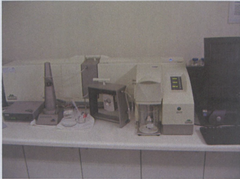
Figure 3.3: Malvern Mastersizer 2000 (Cape Peninsula University of Technology – Rheology laboratory)
