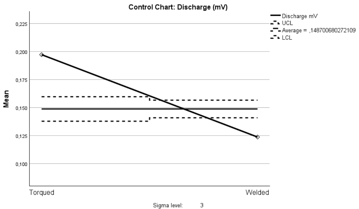
Figure 5.19: Control Chart of Discharge mV (Mean) for Torqued and Welded Packs
