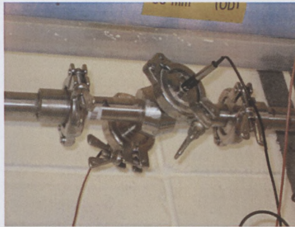
Figure 3.6: Flow adapter (22.5 mm) fitted with two transducers
