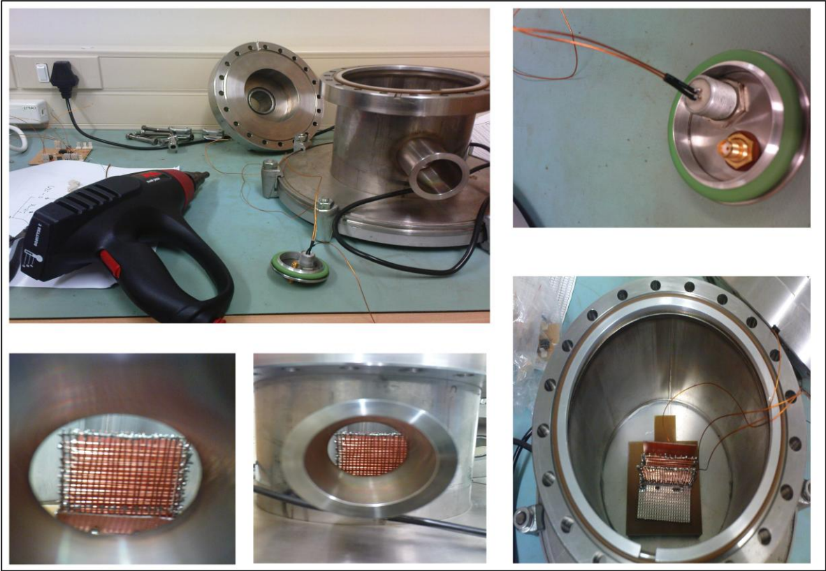
Figure D.1: Photos of the planar sensor development stages
