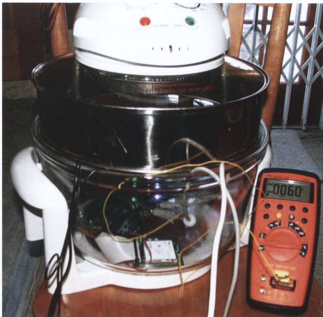
Figure D.1: Gateway and communication module were heated in a small oven to 60°C to verify that the power consumption remained within the 3,5W limit required by the specification.
