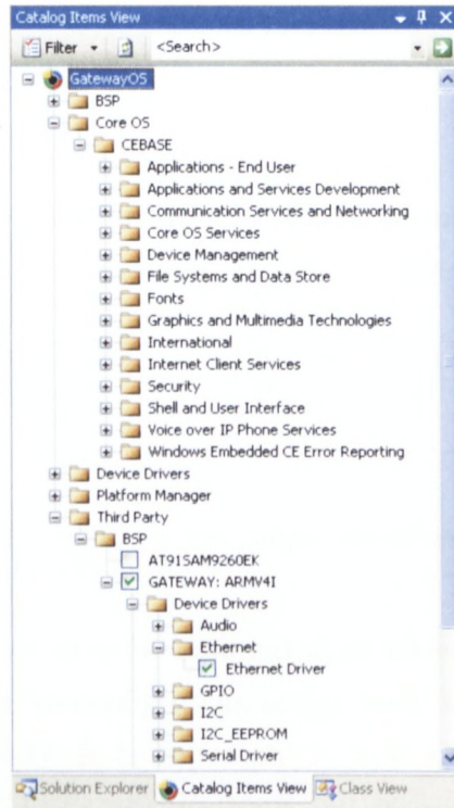
Figure 3.1: The Catalog Items View pane in VS permits the configuration of Windows CE. The BSP for the AT91SAM9260EK was cloned and renamed to GATEWAY:ARMV4I. Shown here is the selection of the Ethernet driver for inclusion in the OS build.
