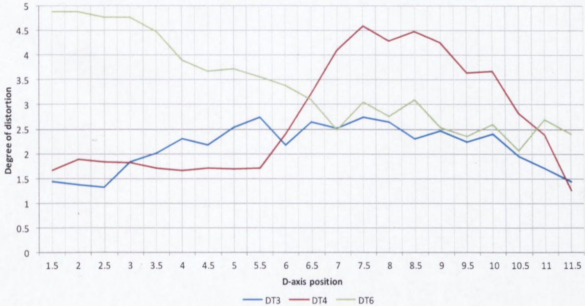
Fig. 3.1.4.6 Distortion of B_l without the 17 th for all d-axis positions
