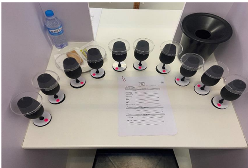
Figure 4.1. Black International Organization for Standardization (ISO 3591:1977) wine-tasting glasses were used during the sensory evaluation sessions.
