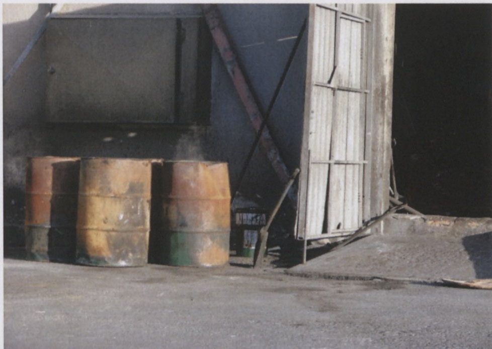
Figure 4.37: Hot bottom ash cooling off while blown into atmosphere
