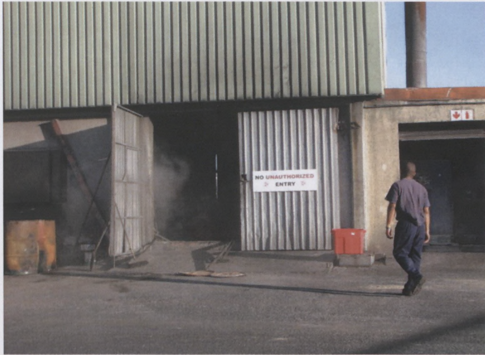
Figure 4.36: Fugitive bottom ash blown into the environment
