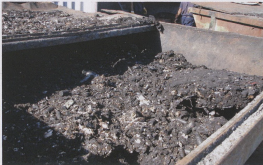
Figure 4.39: Bottom ash partially combusted
