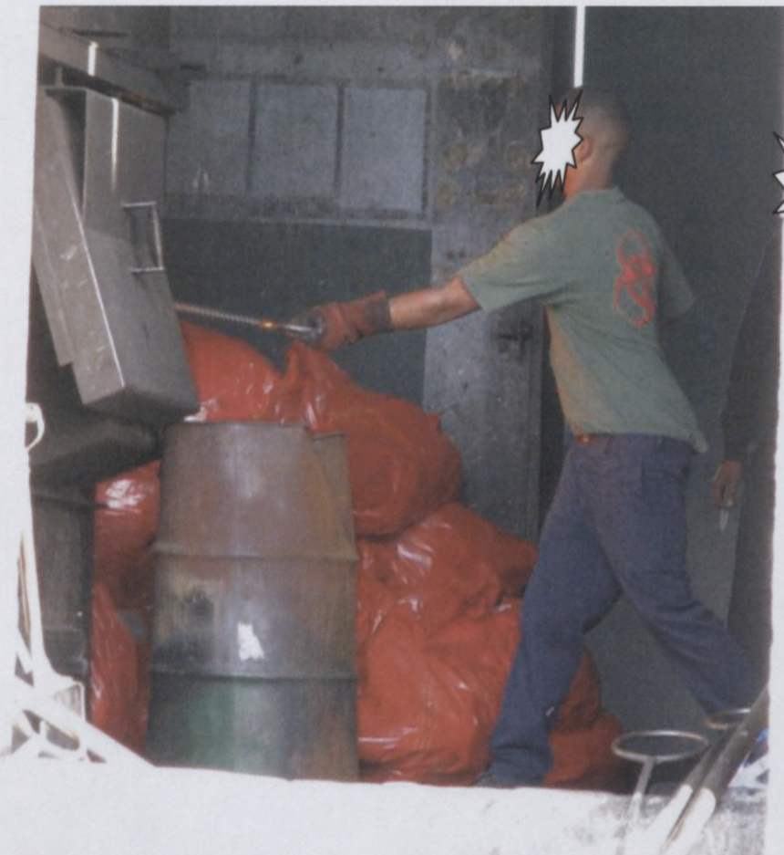
Figure 4.35: Improperly clad workers removing bottom ash
