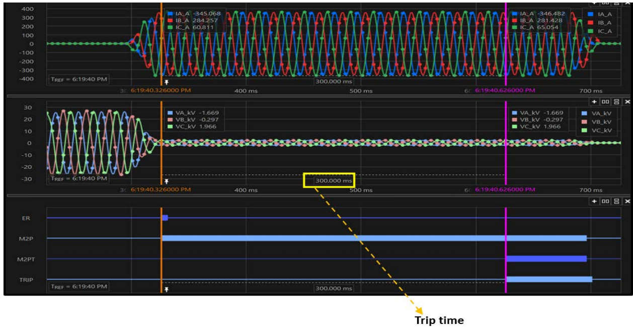
Figure 4.20: Zone 2 three-phase fault events from the relay.
