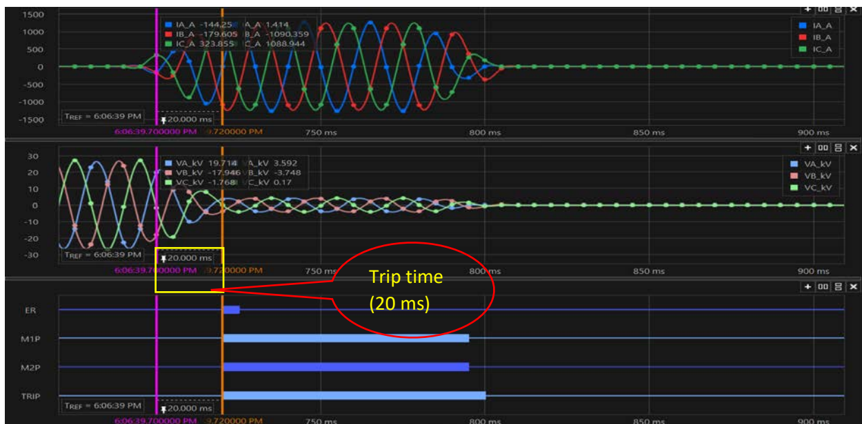
Figure 4.19: Zone 1 three-phase fault events from the relay.
