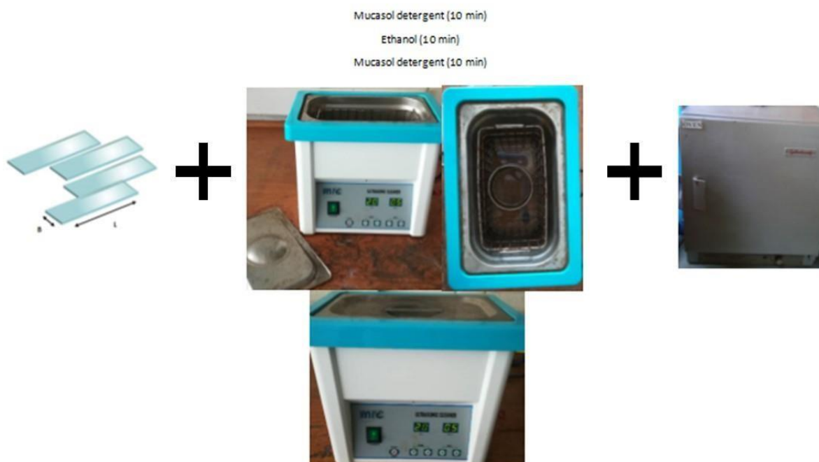
Figure 3. 1: Schematic diagram of the cleaning process of FTO glass
