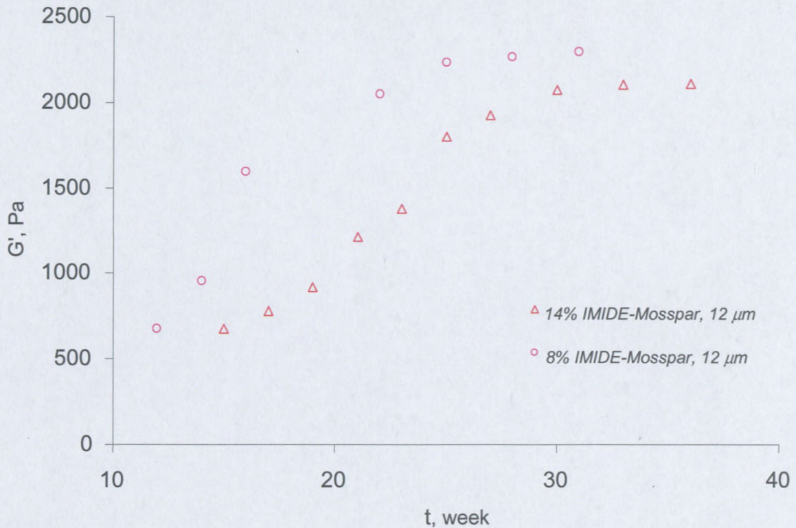
Figure 3.62: Storage modulus vs ageing as a function of surfactant concentration in Mosspar
