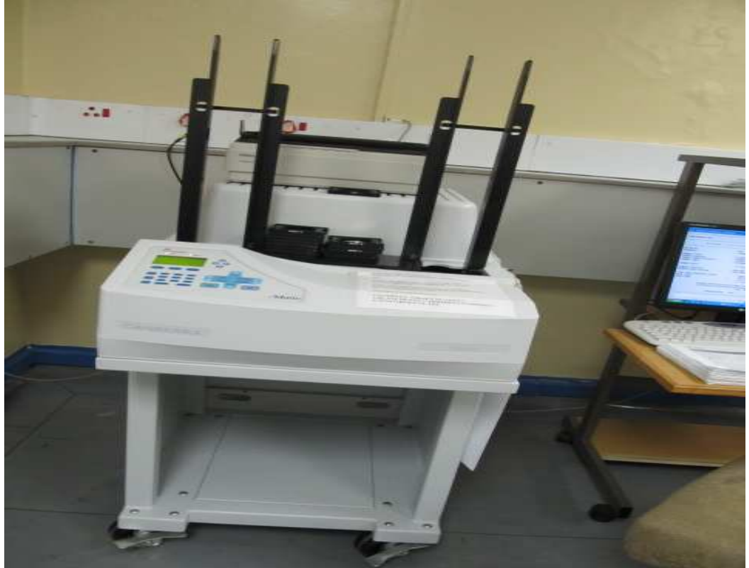
Fig.19. IMatic alpha beta counter as used at KNPS
