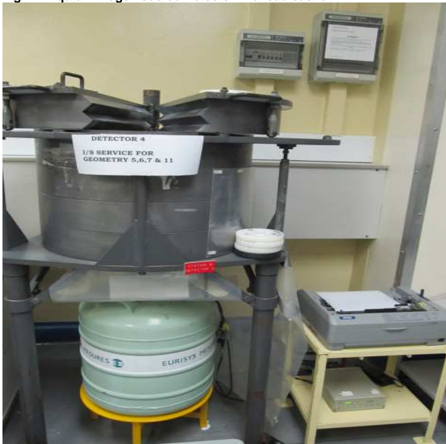
Fig.12. Liquid Nitrogen cooled Detector in a lead castle
