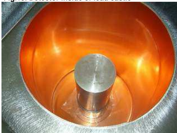
Fig.13. Detector inside of lead castle
