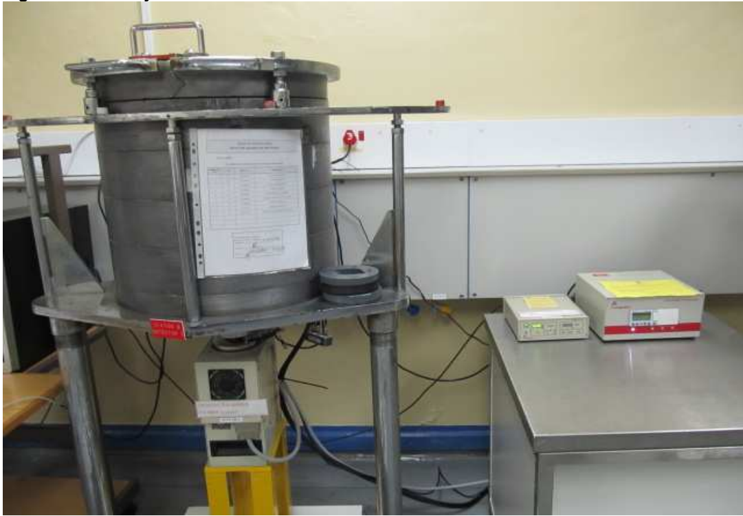
Fig.11. Electrically cooled Gamma detector in a lead castle
