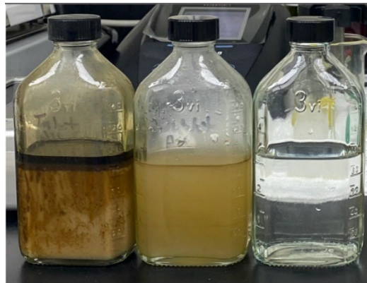
Figure 5.6: Produced water samples showing treatment progression: from left to right, Hydrocyclone Inlet (untreated), Hydrocyclone Outlet/IGF Inlet (partially treated), and IGF Outlet (fully treated).
