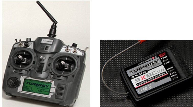
Figure 4. 14: Manual control unit Turnigy 9x 9Ch Transmitter (left) Turnigy 9X8C-V2 8-channel receiver (right)
