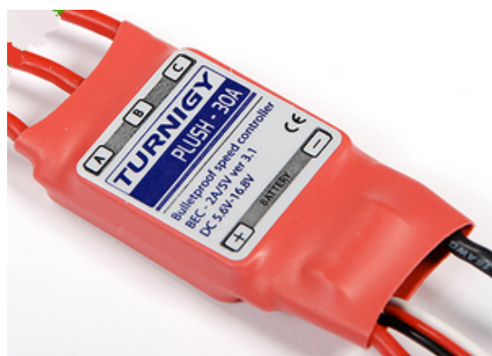
Figure 4. 12: Electronic speed controller
