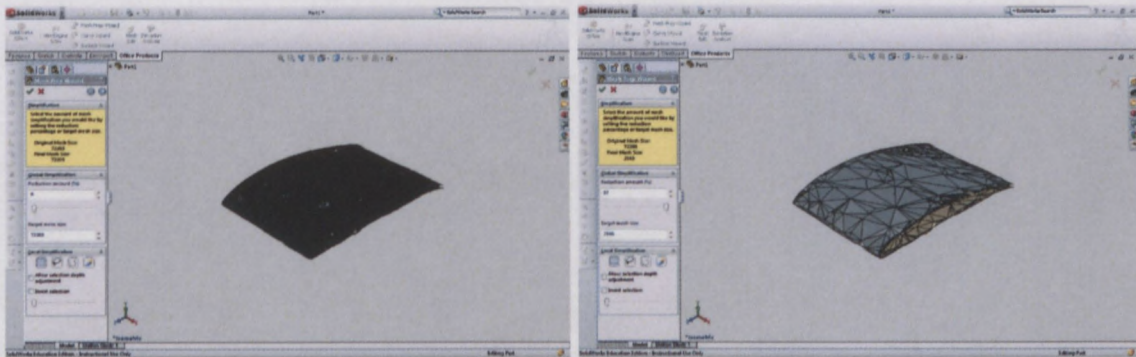
Figure 5.8: Left, before mesh reduction. Right, after mesh reduction.
