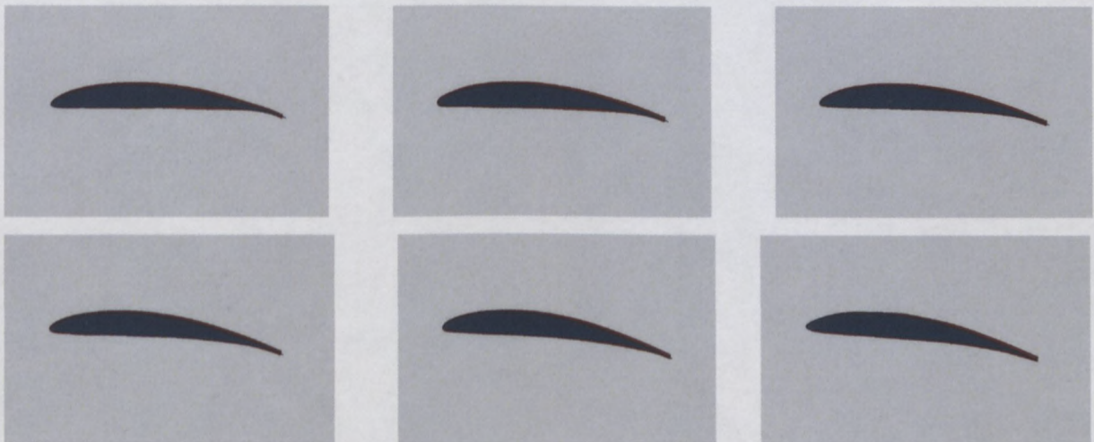
Figure 5.21: Geometrical angles of attack of the flexible section for 5° twist at the different planes. Top left, 3°. Top center, 4°. Top right, 5°. Bottom left, 6°. Bottom center, 7°. Bottom right, 8°.
