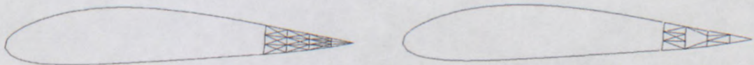
Figure 1.19: Tail section with excess beams in trailing edge (left), optimized trailing edge of tail section (right). (Good, 2003)
