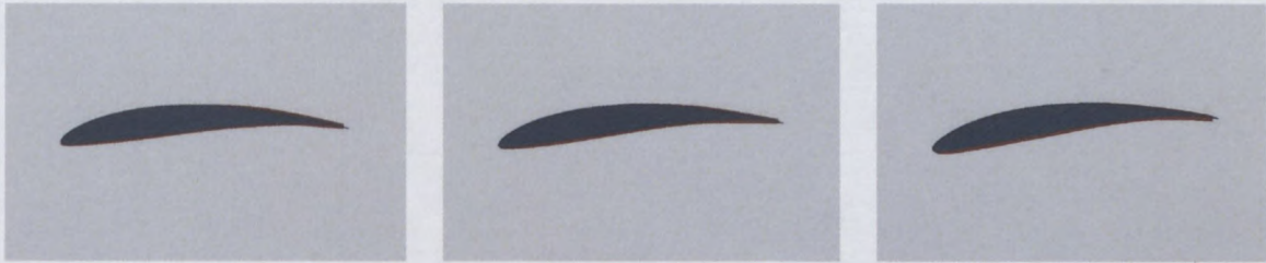
Figure 5.23: Geometrical angles of attack of the flexible section for -9^\circ twist at the different planes. Top left, 3^\circ . Top center, 0.9^\circ . Top right, -0.9^\circ . Bottom left, -2.5^\circ . Bottom center, -4.5^\circ . Bottom right, -6^\circ .
