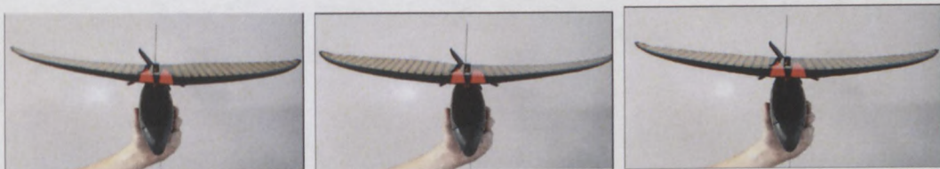
Figure 1.13: Front view of aircraft showing right hand morphing (left), left hand morphing (middle), and neutral position (right). (Lind et al)
