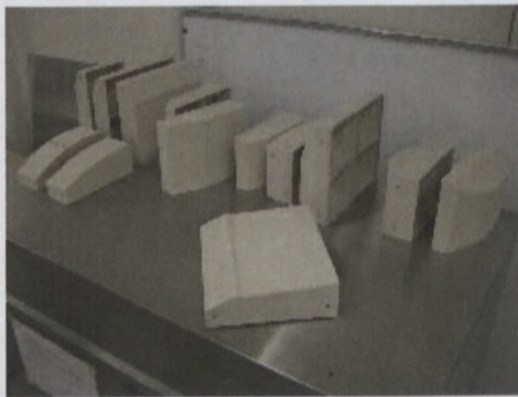
Figure 4.7: The completed mould parts (left), the assembled mould half (right).
