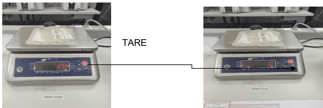
Figure A.2: How to take off the weight of the empty bag
