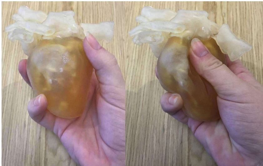
Figure 4.4: 3D printed heart – soft polymers, multi-density single print (by author)
