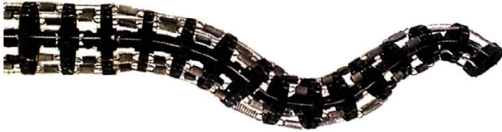
Figure 2.15: Elephant trunk robot incorporating SMA (Trivedi et al., 2008:104)
