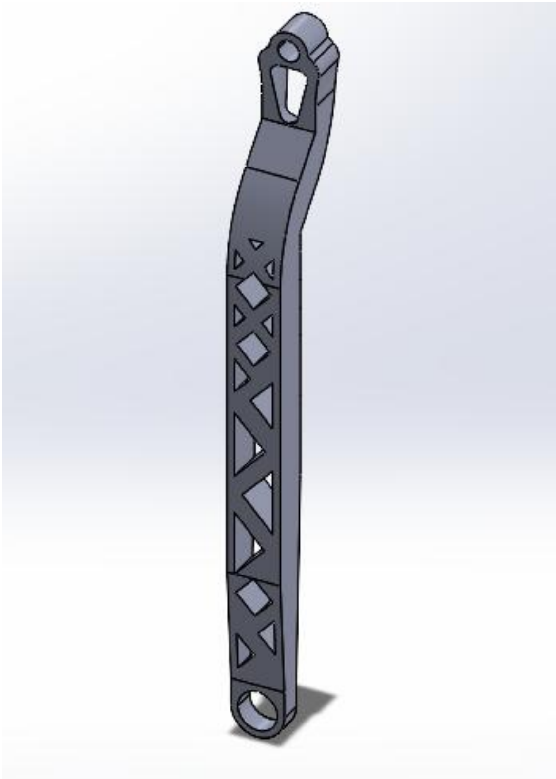
Figure 66: 3D drawing of optimised and refined shank link
