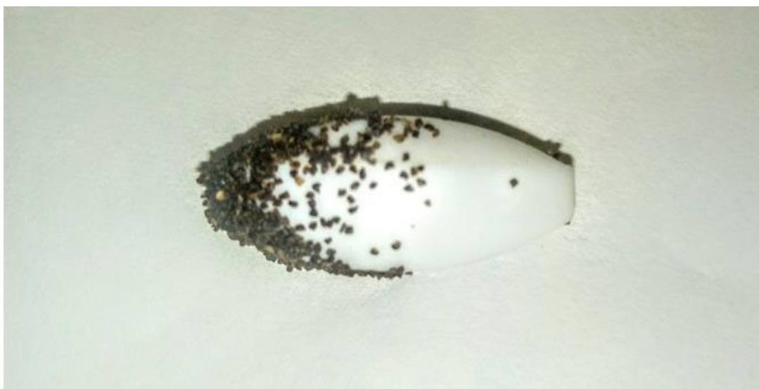
Figure 4.11: Beta-FeOOH/polyamide nanocomposites removed from treated simulated wastewater with an external magnet (Image magnified)
