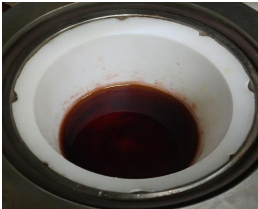
Figure 3.2: The homogenous mixture of water, ethanol and \text{FeCl}_3 \cdot 6\text{H}_2\text{O} inside the Teflon lined reactor
