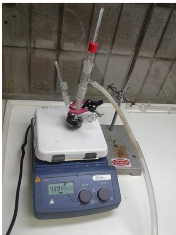
Figure 3.4: Experimental set-up for the synthesis of the \beta -FeOOH/polyamide nanocomposites
