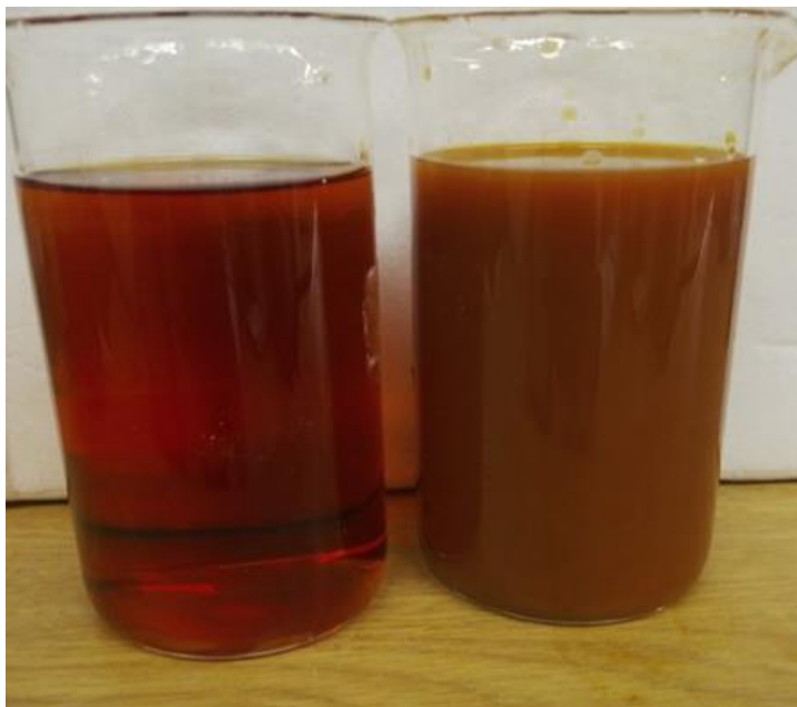
Figure 3.3: Mixture of water, ethanol and \text{FeCl}_3 \cdot 6\text{H}_2\text{O} before introduction into the reactor (left) and solution after 5 h at 100^\circ\text{C} in the reactor (right)
