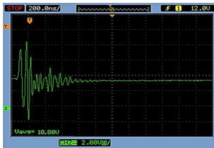
Figure 6-11: Output voltage: current-mode control condition test validation with an input voltage of 3 V
