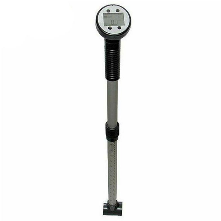
Figure 3.3: A Global water flow probe (YSI, Yellow Springs (OH), United States)
