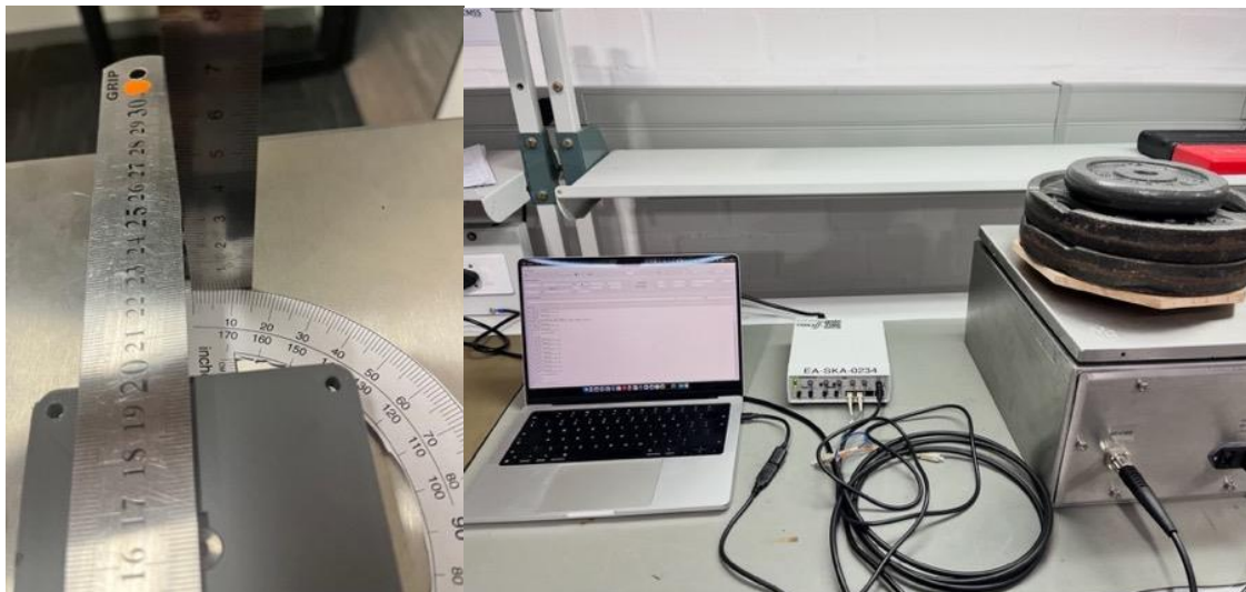
Figure 6.4: Angular accuracy measurements and loaded test in progress.
