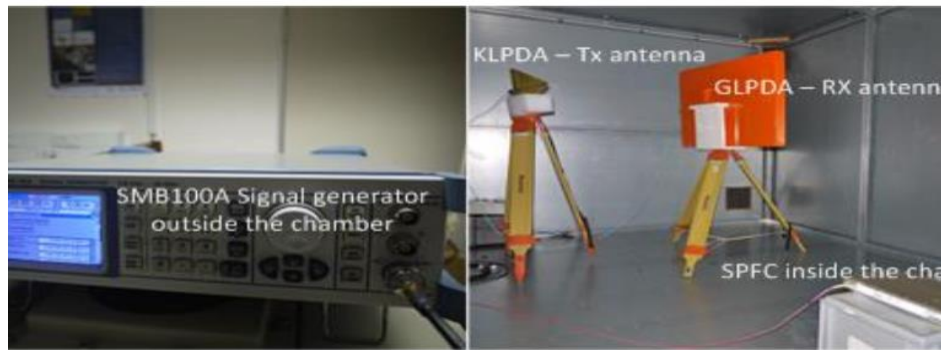
Figure 2.10: Susceptibility test setup. (from Smit, 2020).
