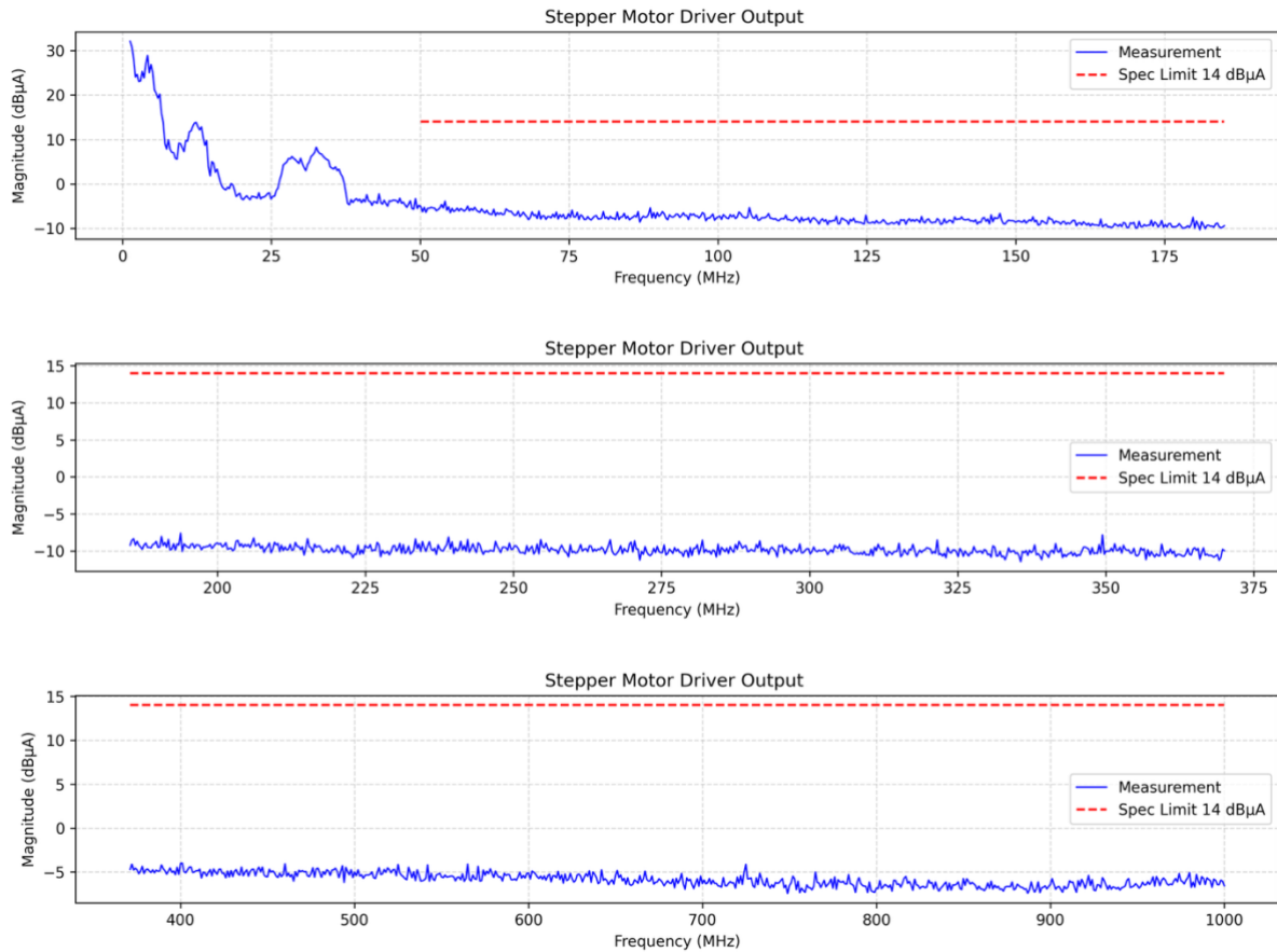
Figure 6.20: Stepper motor driver output cable CMC results.
