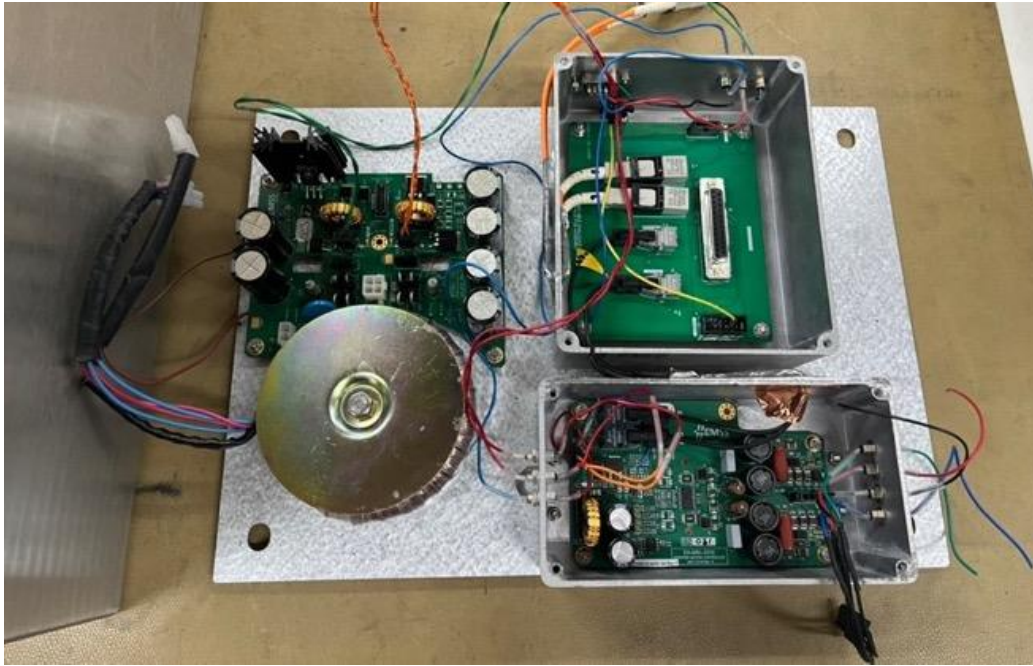
Figure 5.5: Mounting of subsystems to mounting plate.
