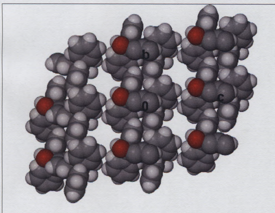
Figure 3.31 Space filled diagram for H·2DMF viewed along [100]. The guest molecules reside in the open channels (the guests are omitted).
