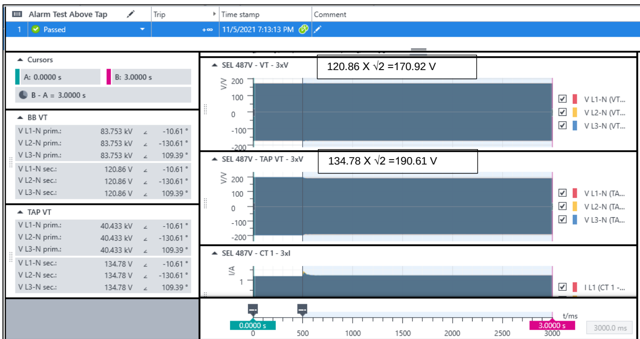
Figure 6.9. RelaySimTest simulation voltage waveforms for three element failures above the tap
