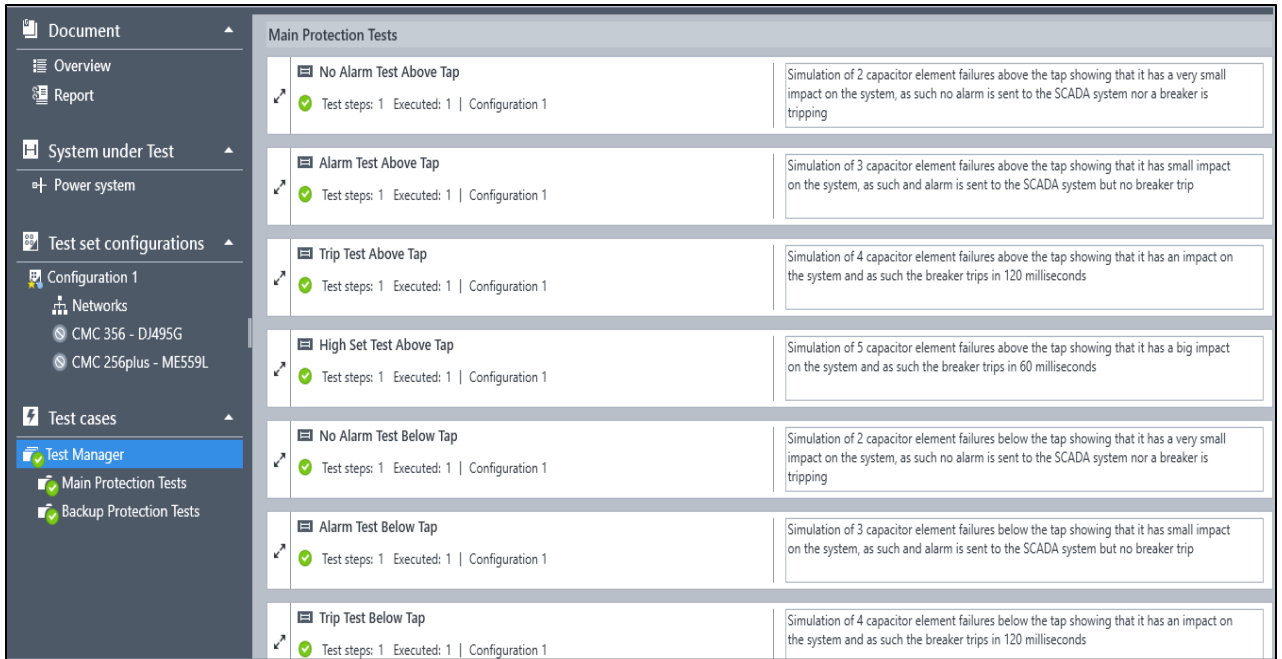
Figure 6.3. RelaySimTest successful execution of test cases
