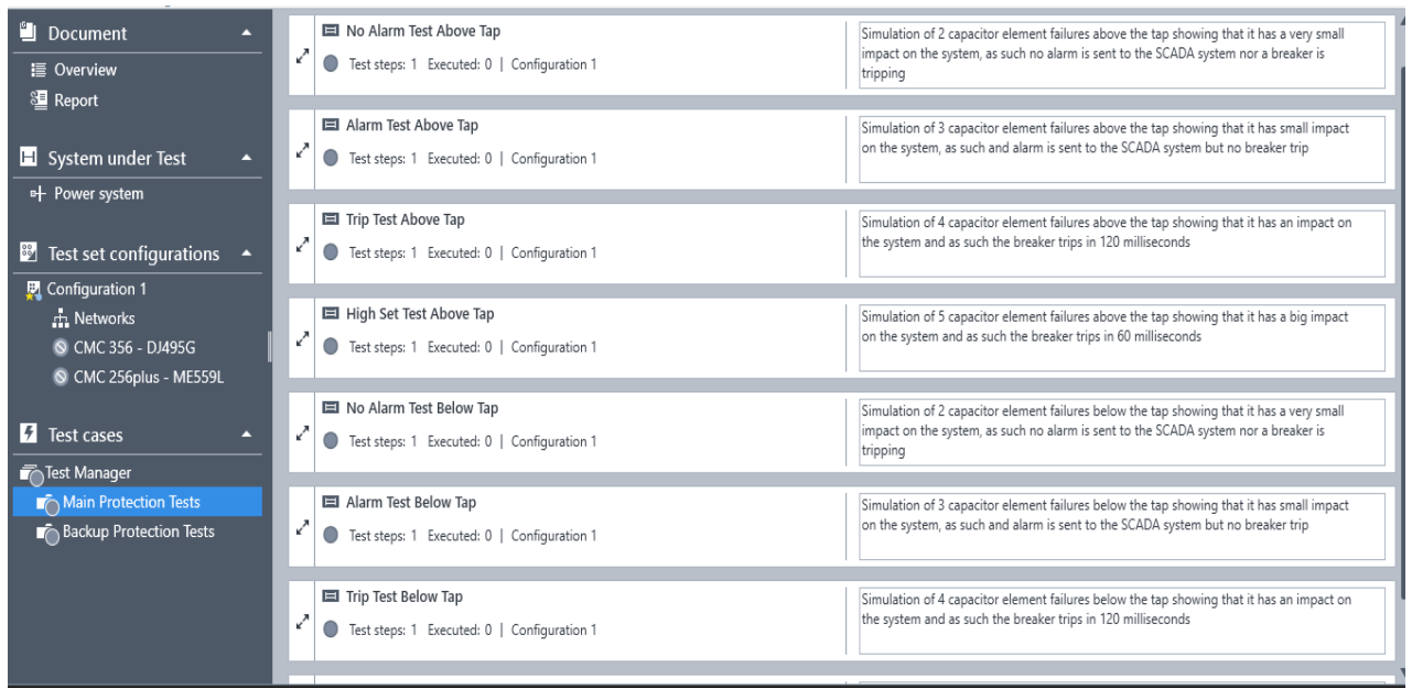
Figure 5.50. RelaySimTest main test cases configuration
