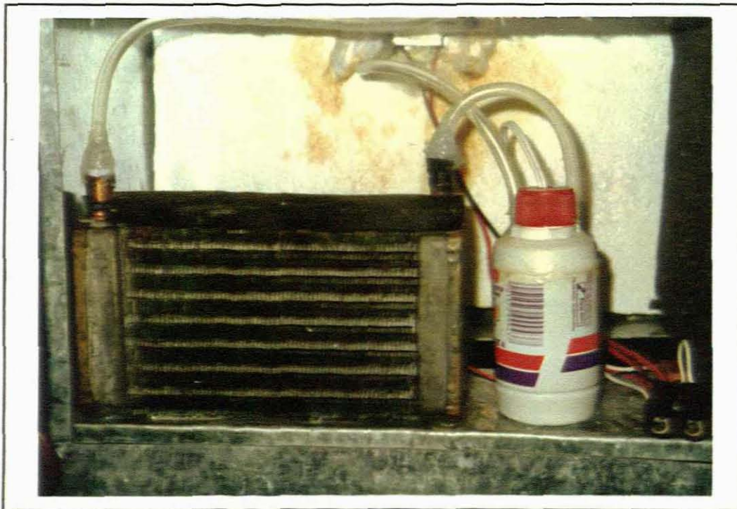
Figure 4.5 The heat exchanger used in the prototype coolerbox. The water pump is situated inside the plastic water container.
