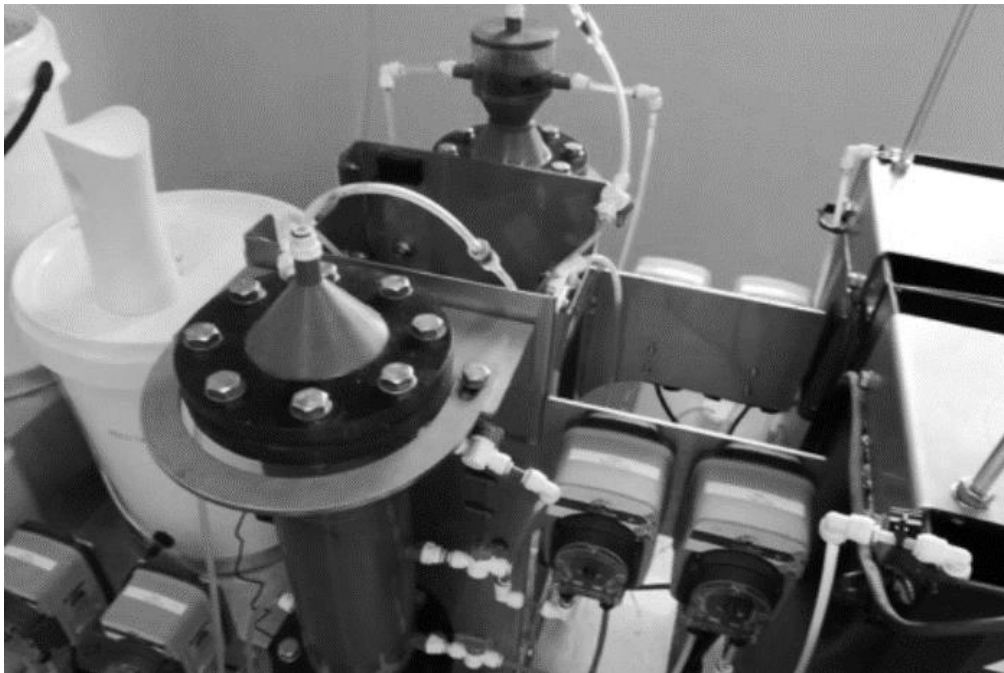
Figure 7. Lab-Scale Treatment Plant for PSW [21]– Reprinted from Membranes, vol 11, Meyo, H.B.; Njoya, M.; Basitere, M.; Ntwampe, S.K.O.; Kaskote, E., “Treatment of Poultry Slaughterhouse Wastewater (PSW) Using a Pretreatment Stage, an Expanded Granular Sludge Bed Reactor (EGSB), and a Membrane Bioreactor (MBR)”. Copyright (2021), with permission from MDPI.
