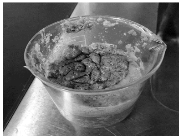
(b) Collected coagulated FOG after pre-treatment
